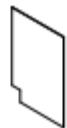
BSPR - (23 3/4" x 34 1/2" x 3/4") BSPL - (23 3/4" x 34 1/2" x 3/4") VSPR - (21" x 34 1/2" x 3/4") VSPL - (21" x 34 1/2" x 3/4")
